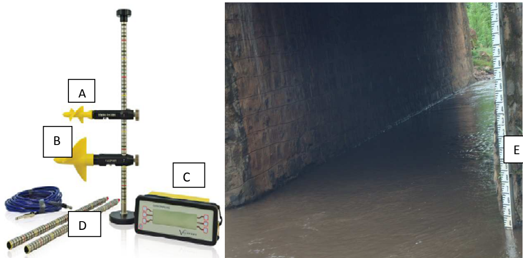
Figure 7: Current Meter model used for measuring river flow and staff gauge (E) at DR monitoring station
