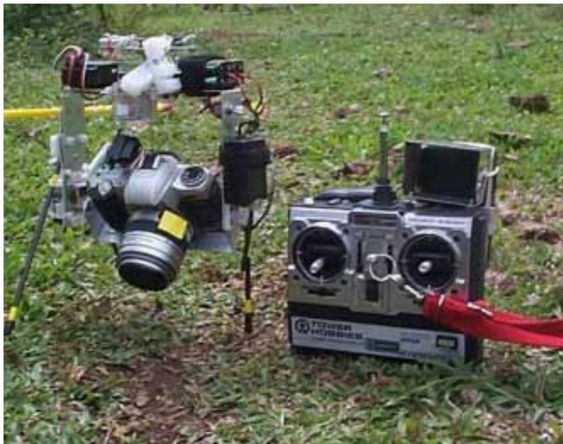
Figure 30. The image shows the camera setup, consisting of the remote control unit and a 35-mm film-based camera with cradle. The system can also be flown with a high-resolution digital camera, and is airborne using various kite and balloon platforms, depending on wind conditions.
