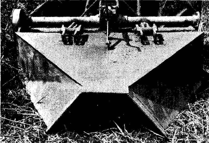
**Photo 3: Levee maker designed and fabricated by CIAT personnel.**
