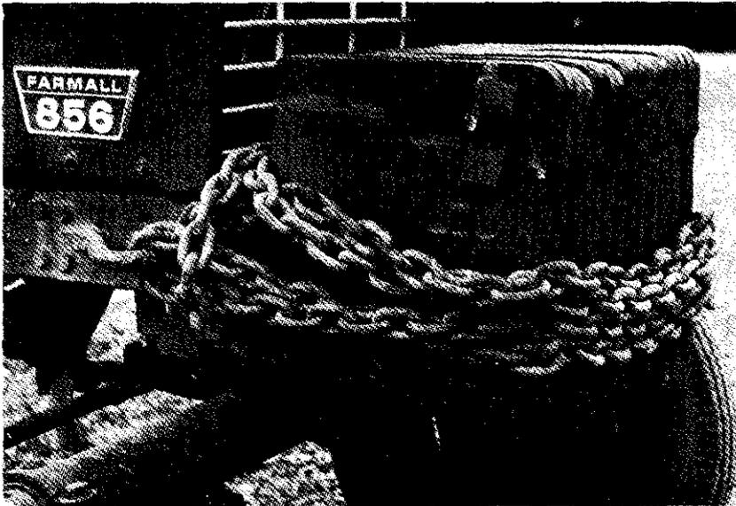
**Photo 1: Front weights, chain and pull points to stabilize the tractor and for pulling when stuck in the mud.**
