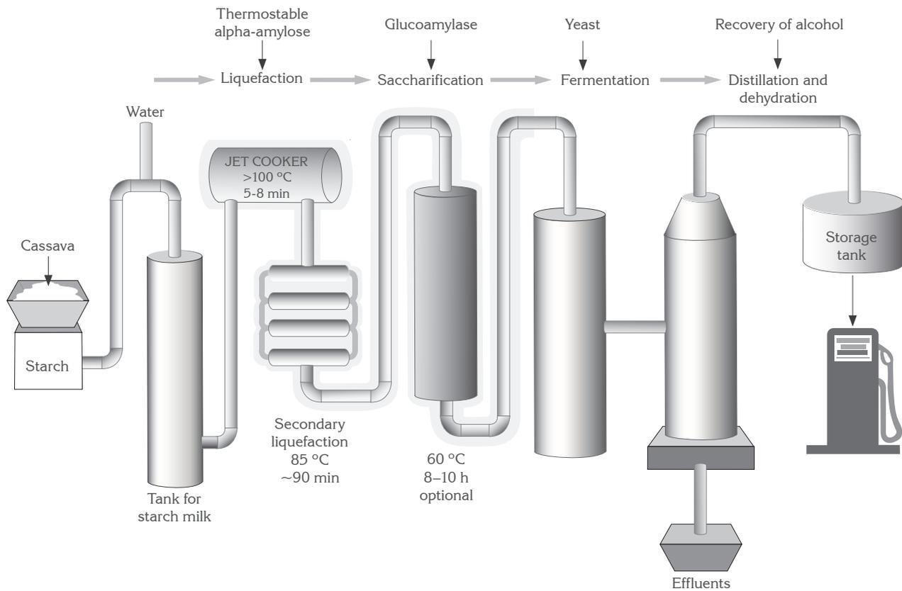
Figure 24-6. Conventional process for producing bioethanol from cassava (from Genencor International, a Danisco company; see [www.genencor.com](http://www.genencor.com)).
