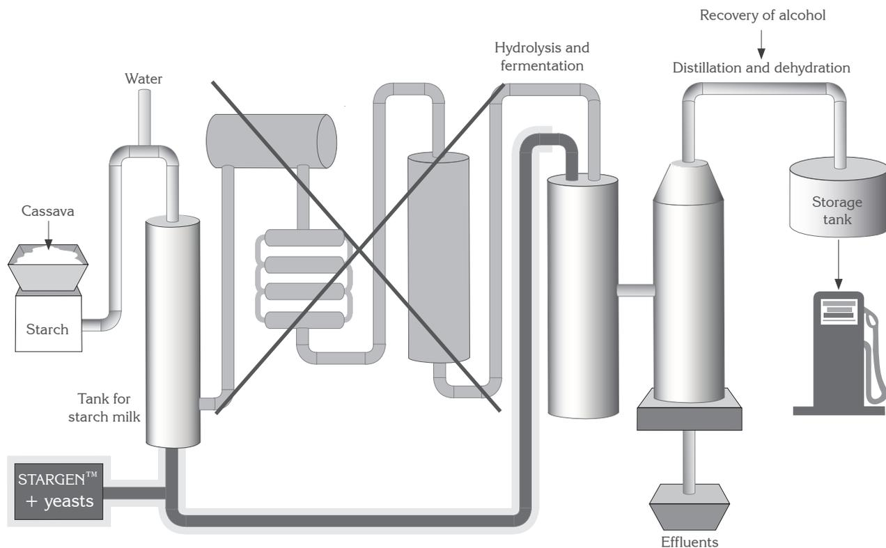
Figure 24-7. Simultaneous hydrolysis and fermentation (SHF) (from Genencor International, a Danisco company; see [www.genencor.com](http://www.genencor.com)).
