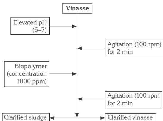
Figure 24-9. Sequence of clarification of vinasse, using biopolymers.
