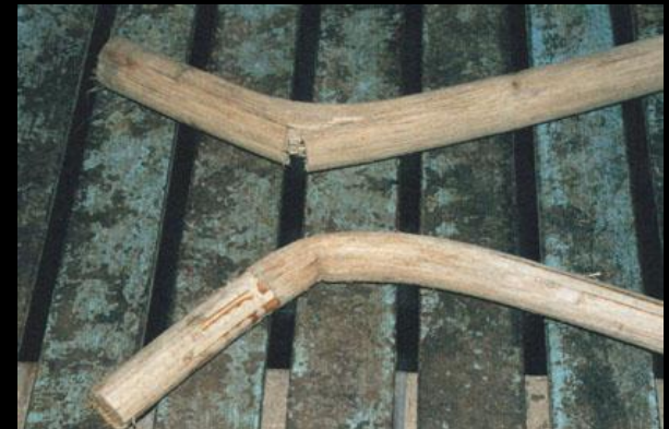
Right: Split and cracked poles due to improper bending.
