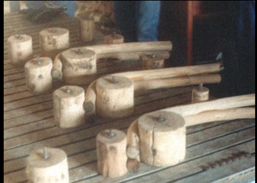
Photo: Steamed poles awaiting bending in jigs
