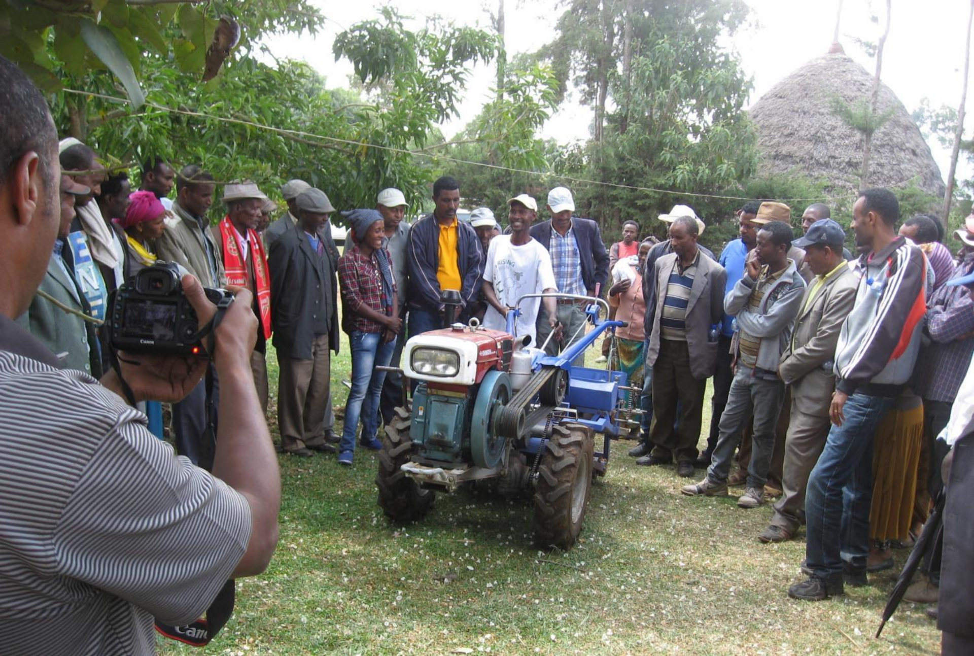
A trained farmer in Jawe kebele demonstrates how a multipurpose two wheel tractor provides water pumping and seeding services, and transports produce from the farm
