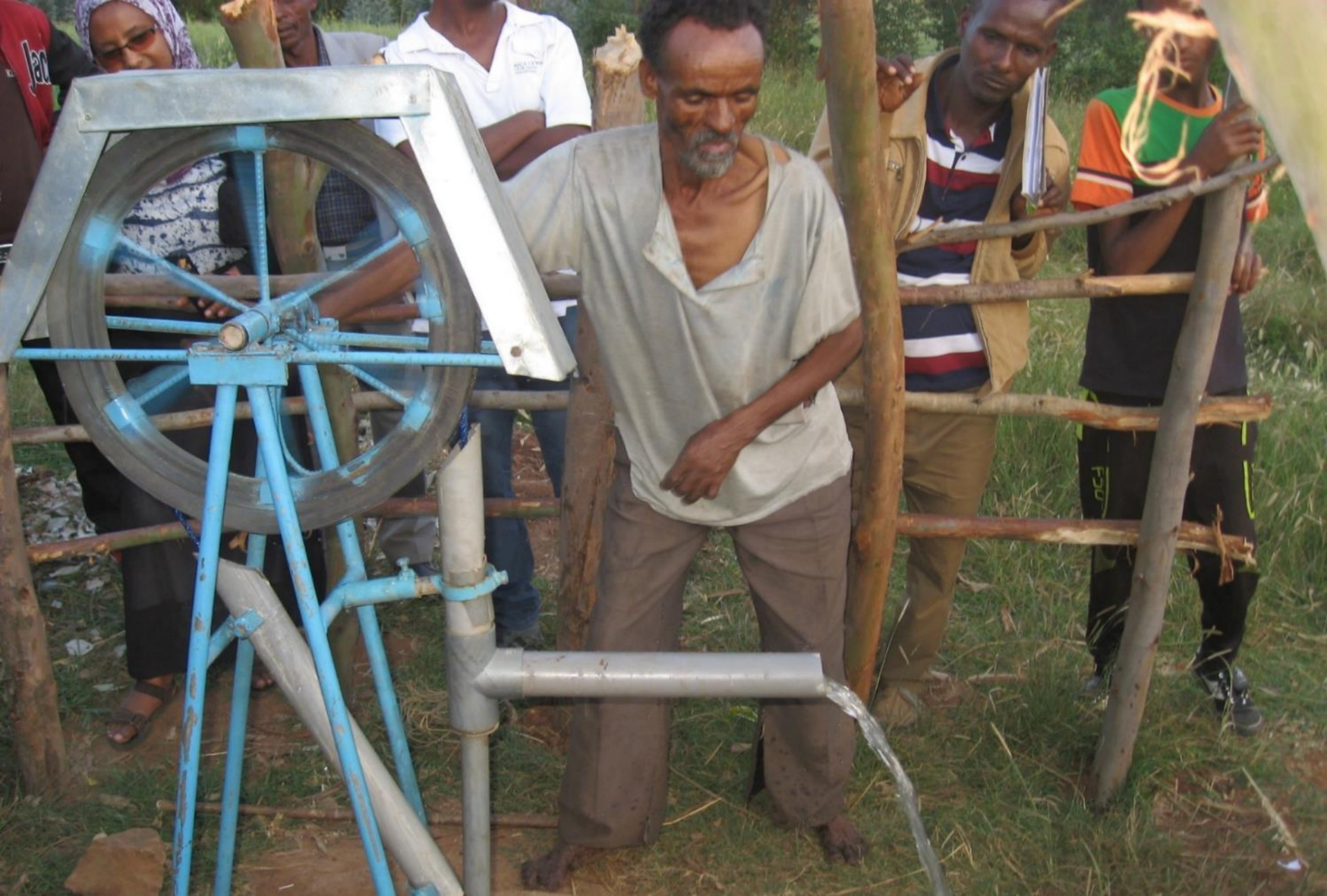
A rope and washer pump installed on shallow wells in Upper Gana kebele – It helps to irrigate vegetables and fruit trees, and pump water for livestock
