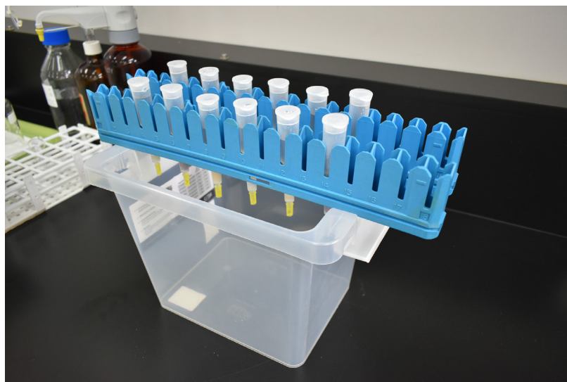
Figure 12. Ion exchange cartridges position in a rack (with the bottom closed with a cap)
