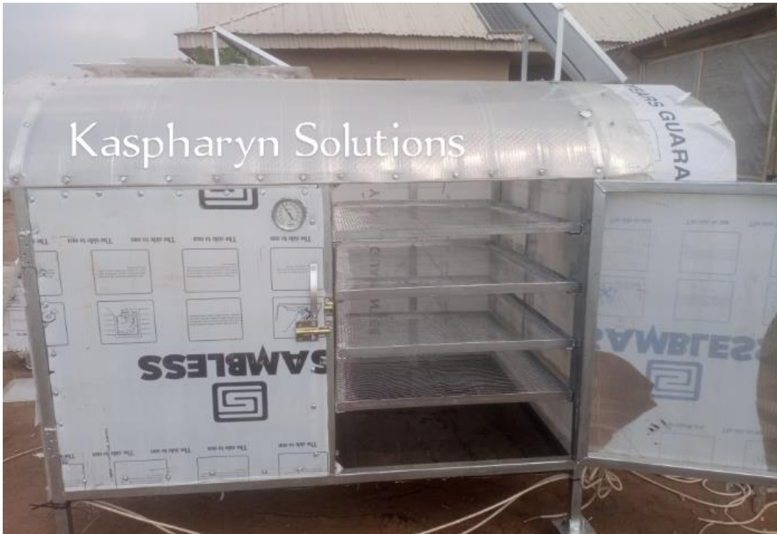
Figure 7: The Hybrid Food Sun-dryer
