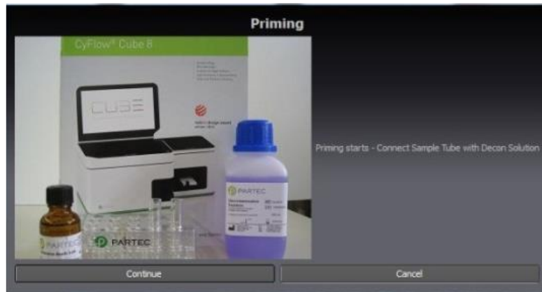
Figure 7. Step 1 of the priming process.
