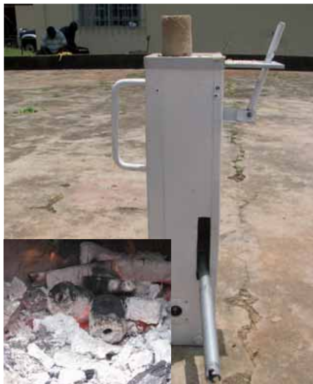
The Cameroonian briquette-maker and the briquettes in use (inset) in the improved parboiling stove
