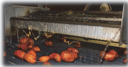
Fungicide application using a waterfall curtain
