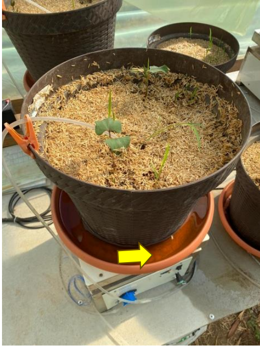
Figure 8. Lysimeter applying excessive irrigation
