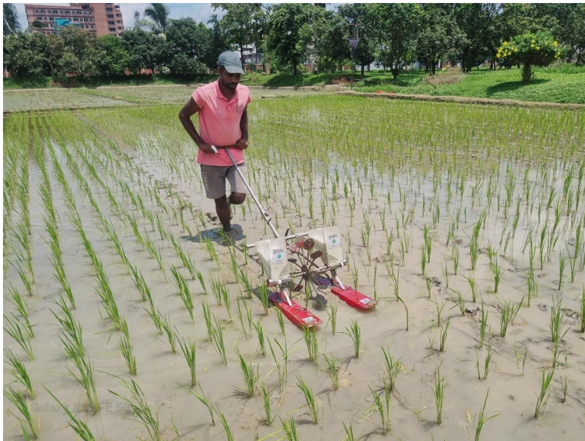
Photo 4: Prilled urea deep placement by using the BRRI-developed urea deep placement applicator. Photo credit: Kamruzzaman Milon, BRRI
