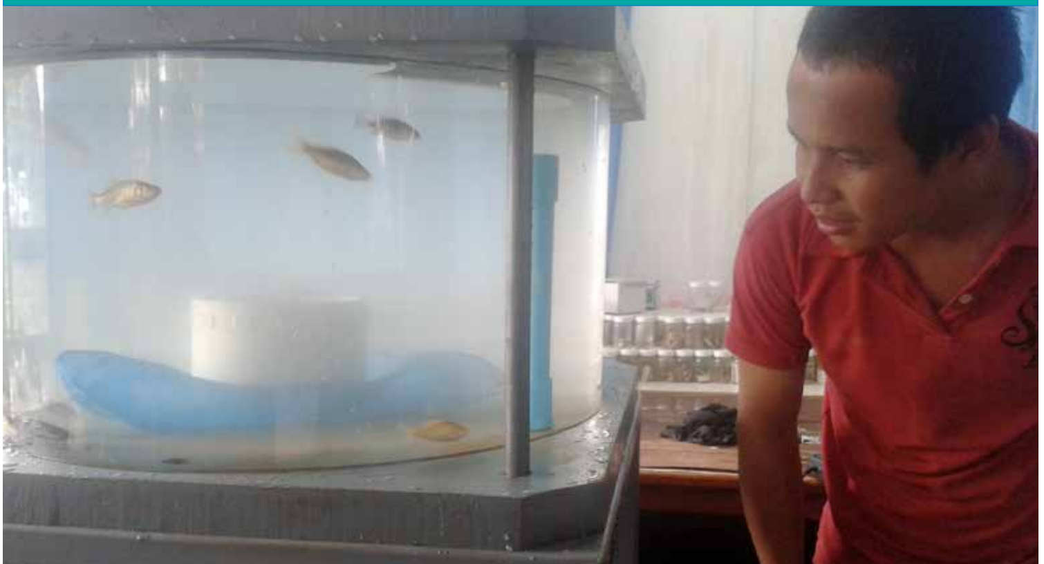
A Lao university researcher observing fish in a barotrauma chamber, where they will be subjected to a rapid pressure change similar to what they would experience as they pass downstream through a hydro turbine. Photo: Garry Thorncraft
