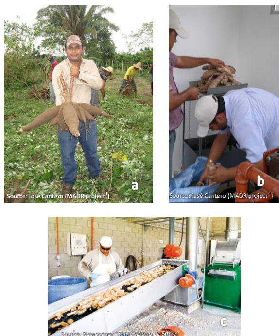
Figure 2 (a) Cassava harvest in Cordoba, Colombia 1 ; (b) weighing cassava at the “Almidones de Sucre (AdS)” plant to estimate starch content; (c) cassava cutting as the initial process in the AdS factory.
