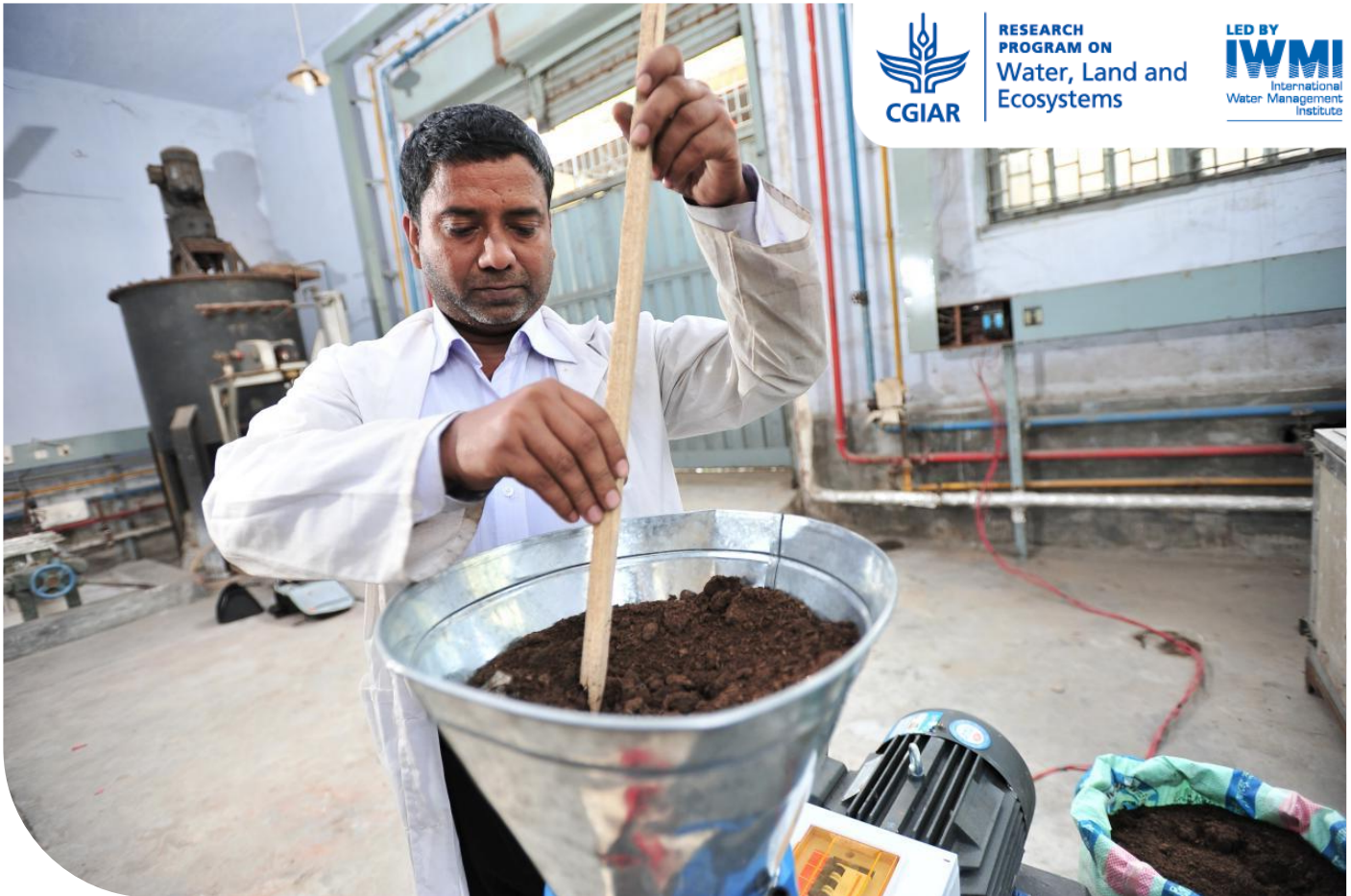
Turning processed human waste into safe fertilizer pellets. (Neil Palmer/CIAT)
