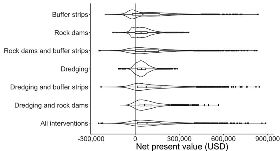
Fig. 7. Distributions of projected outcomes of decisions to implement dredging, rock dams and buffer scheme interventions, as well as all their combinations, to reduce sedimentation in the Lagdwenda reservoir in Burkina Faso.
