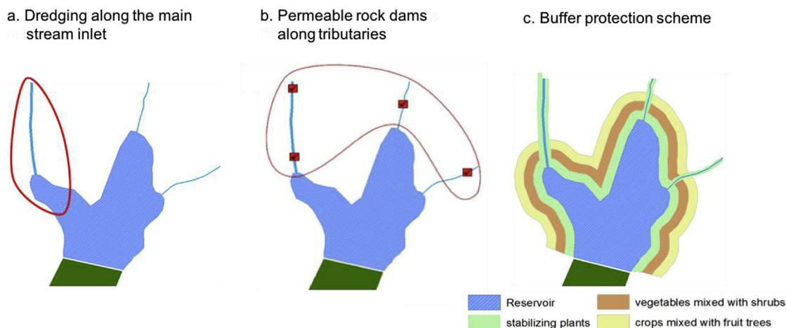
Fig. 4. Intervention options to reduce sedimentation in the Lagdwenda reservoir in Burkina Faso, co-designed by workshop participants: a. dredging for 2 km along the main stream inlet to a depth of 3 m; b. low dams of loose stone retained by mesh wire every 5 km along the stream network upstream of the reservoir; c. three buffer strips of 75–100 m each.
