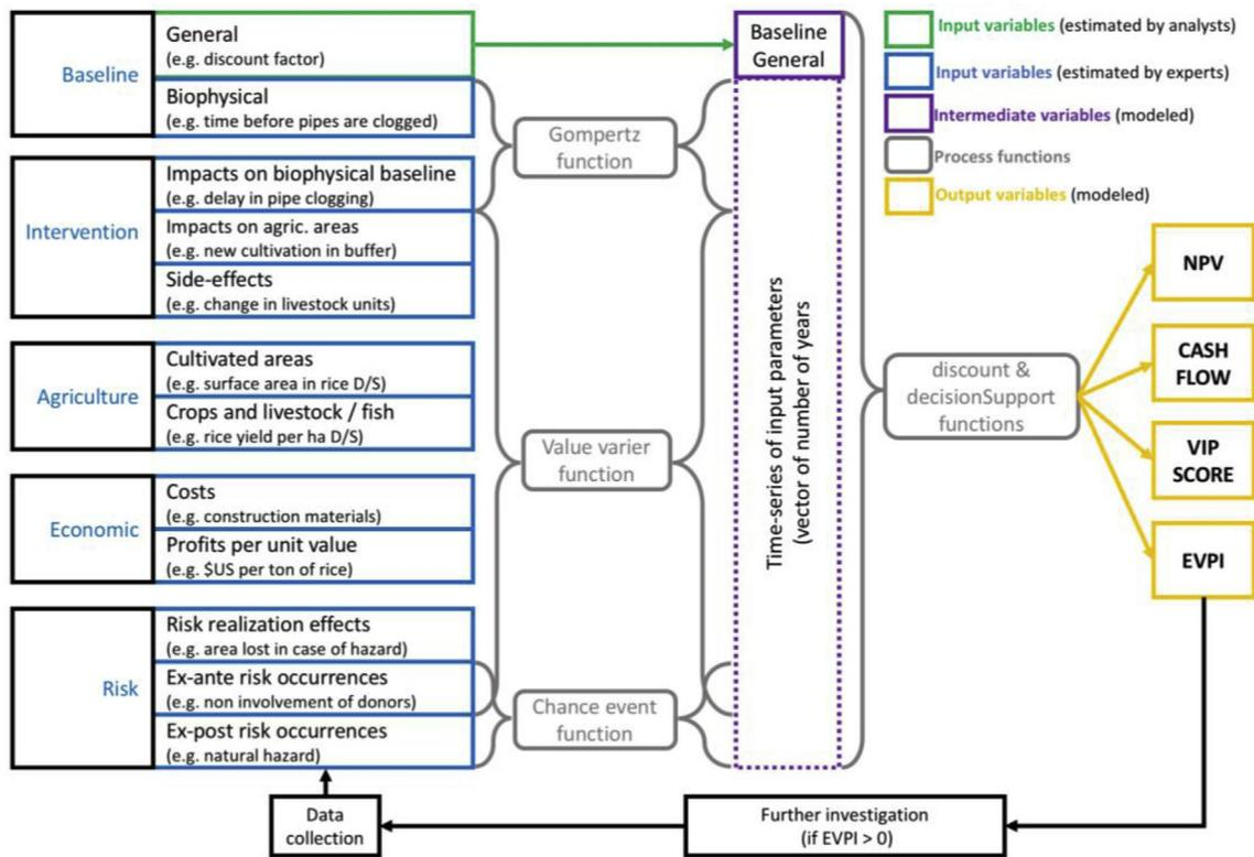
Fig. 6. Input-Output diagram of the simulation model of decisions to implement dredging, rock dams and buffer scheme interventions, as well as all their combinations, to reduce sedimentation in the Lagdwenda reservoir in Burkina Faso. Process functions are detailed in Step 3.
