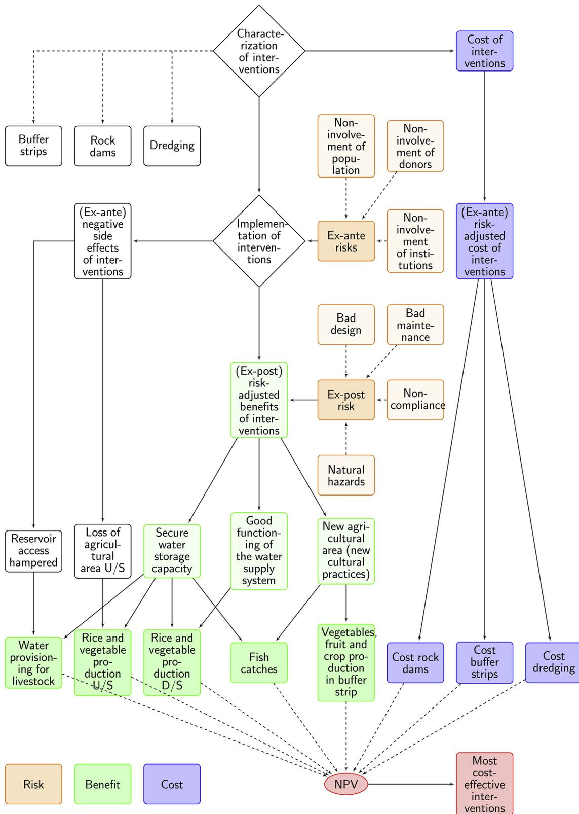
Fig. 5. Diagram of the overall model structure of interventions to reduce sedimentation in the Lagdwenda reservoir in Burkina Faso. NPV is the Net Present Value for all interventions. D/S = downstream; U/S = upstream.
