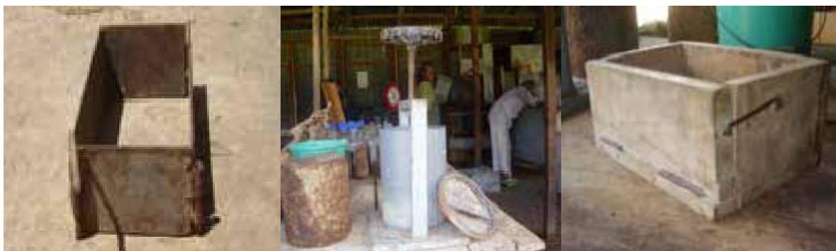
Figure 3.61 Moulds made from metal sheets, tubes, wood.
