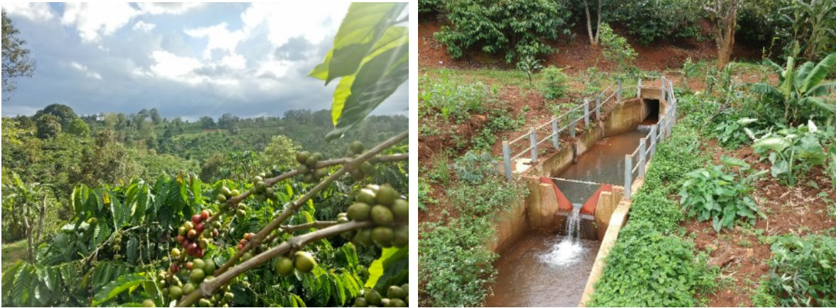
Pictures 1 Left: Overview of the experimental catchment. Right: the V-notch gauging station
