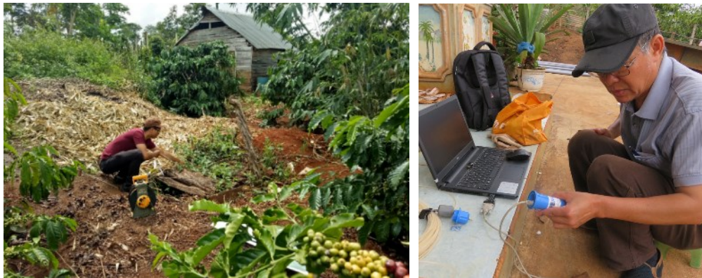
Picture 4 left: A field expert from HRNS surveys groundwater levels – right: Programming groundwater level loggers
