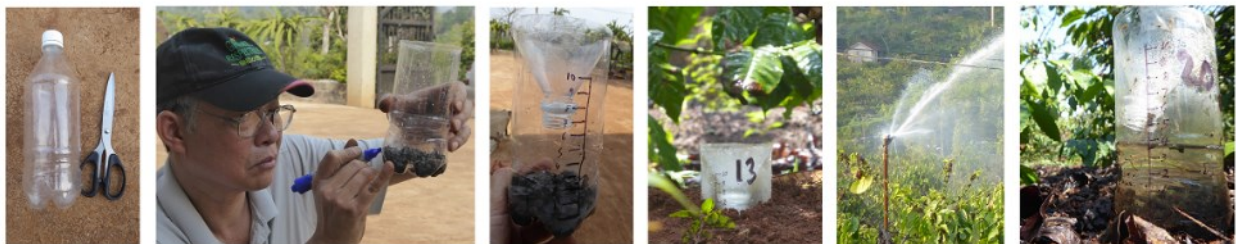
Picture 8 - steps to create catch-cans for measuring sprinkler uniformity
