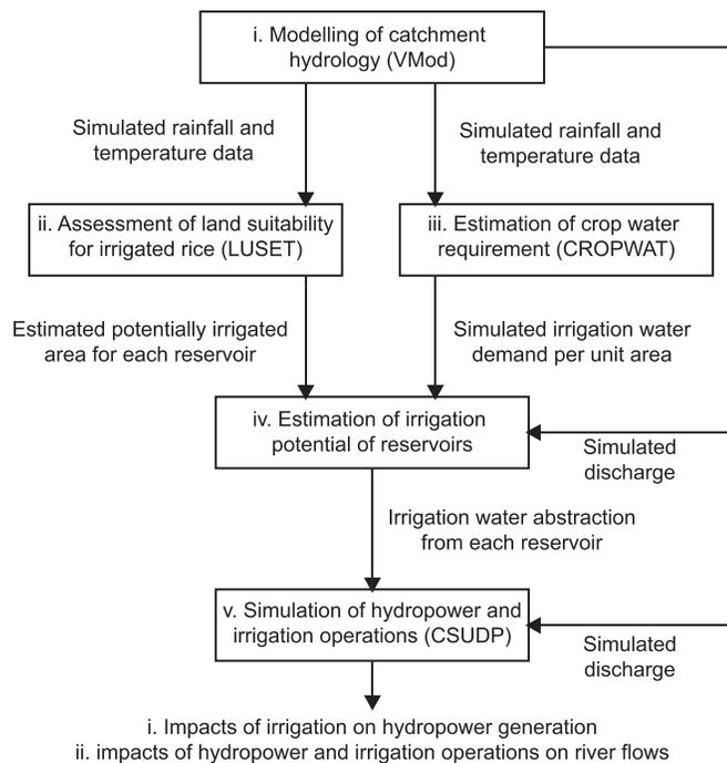
**Fig. 2.** Stages of the developed modeling approach and their relationships in the assessment of irrigation potential of a cascade of multipurpose reservoirs and their river flow impacts; a detailed description of modeling stages is presented in Section 1 of the Supplemental Data
