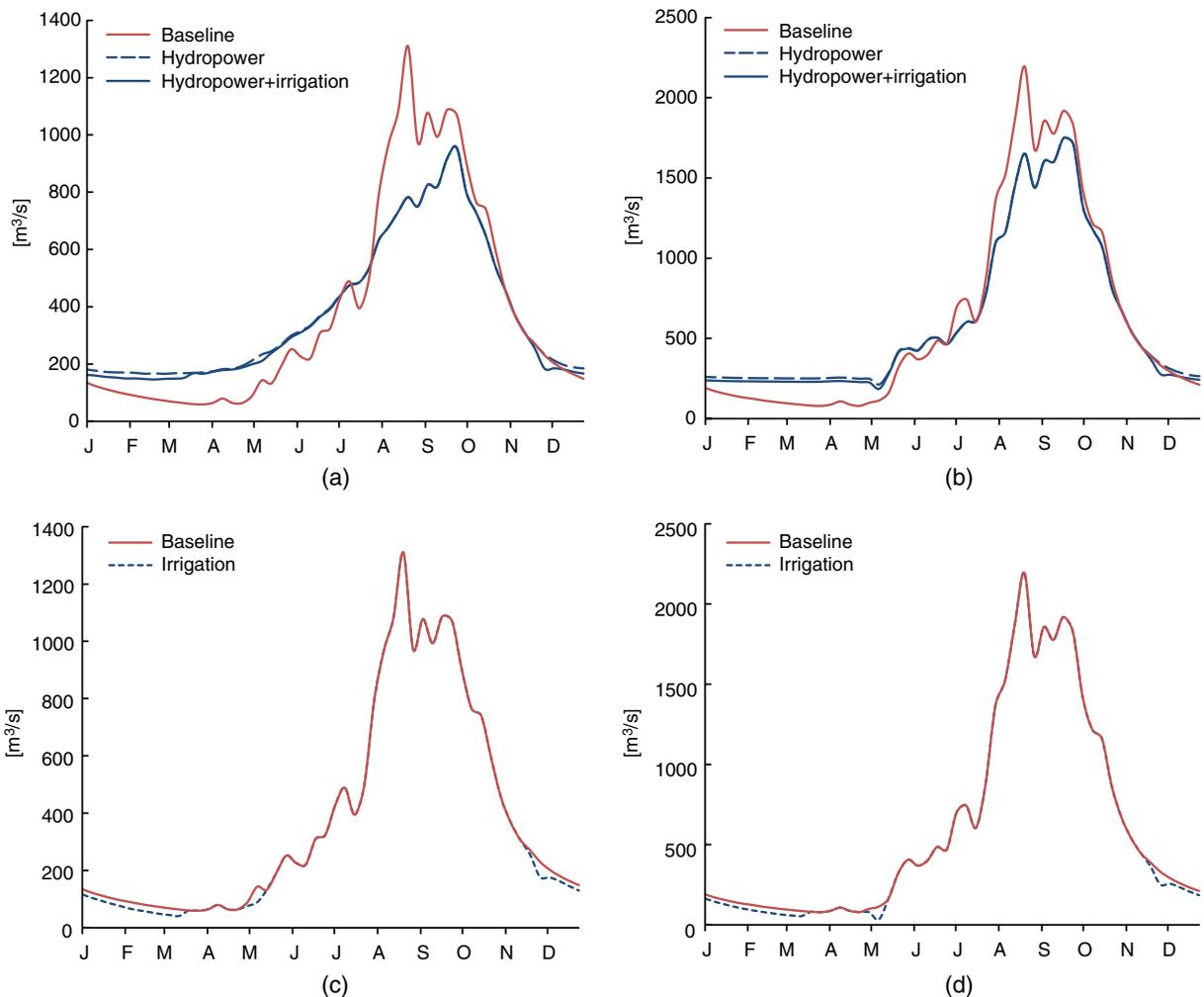
**Fig. 4.** Average river flow impacts at the border of Vietnam and Cambodia (immediately downstream Sesan 1 dam) and at the outlet of Sesan Catchment over the period 2002–2006: (a, b) impacts of hydropower and combined hydropower and irrigation; (c, d) impacts of irrigation on baseline flows (i.e., natural nonregulated flows)
