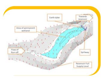
The dyke and spillway would need to be designed to survive complete inundation for part of the year. The wetlands would also trap sediment, a bonus for dam operator. The wetland would eventually mature into a productive marsh.
