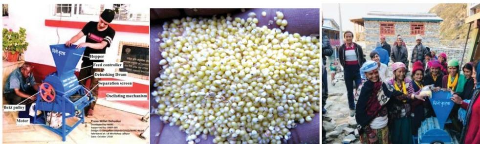
**Figure 2.** Electric proso millet dehusker testing at Khumaltar and field testing in Humla.
