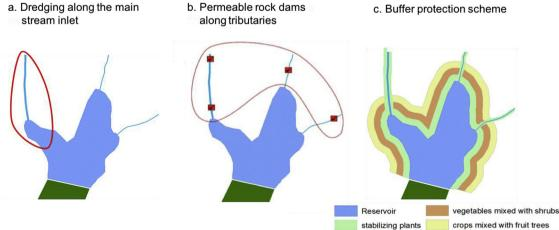
Fig. 4. Intervention options to reduce sedimentation in the Lagdwenda reservoir in Burkina Faso, co-designed by workshop participants: a. dredging for 2 km along the main stream inlet to a depth of 3 m; b. low dams of loose stone retained by mesh wire every 5 km along the stream network upstream of the reservoir; c. three buffer strips of 75-100 m each.
