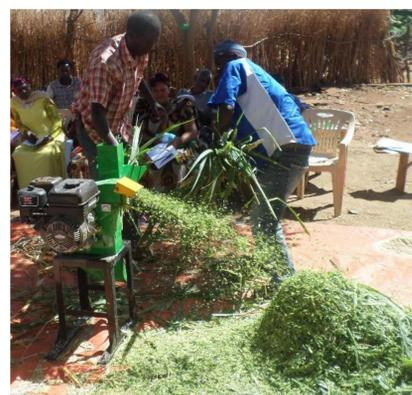
Figure 1: A forage chopper in action
