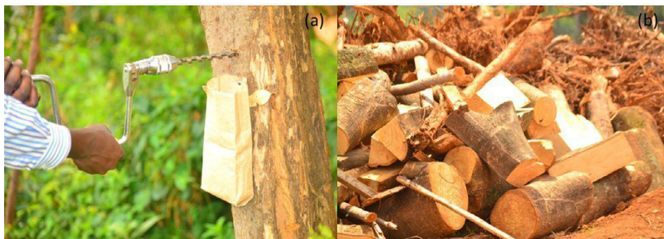
Fig. 2. The two methods for wood density sampling (a) Auger method involving coring the tree trunk (b) conventional destructive method involving cutting discs.
