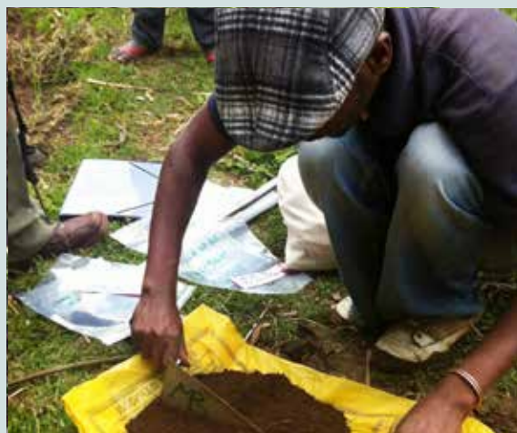
(b) Soil subsampling via coning and quartering
