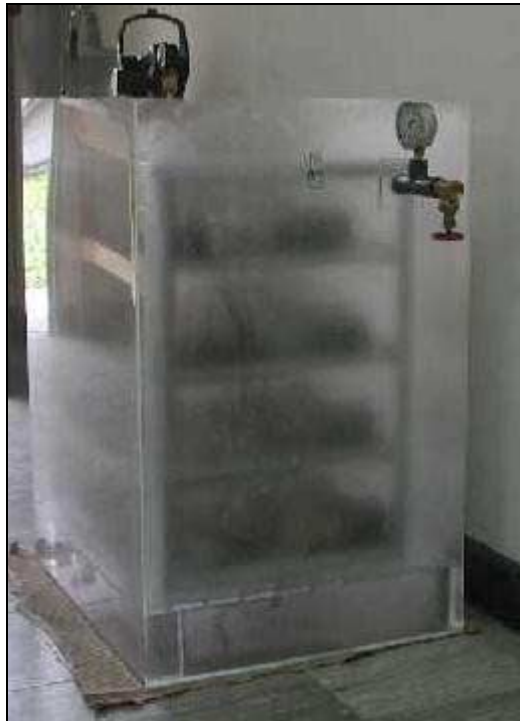
Figure 2.15. A chamber for controlled atmospheres designed to carry out applied research on the control of postharvest physiological deterioration in cassava.
