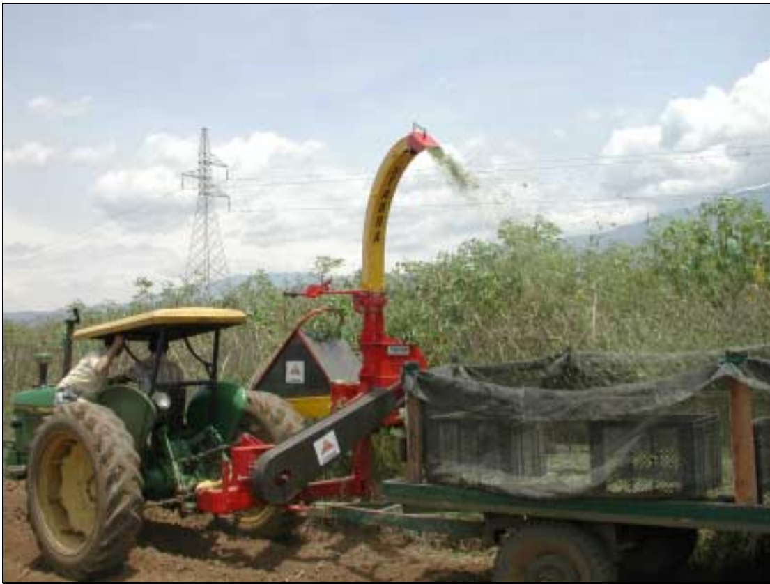
Figure 3.1. The foliage mechanical harvester in action. Cassava tender canopy is cut and stored in a trailer.
