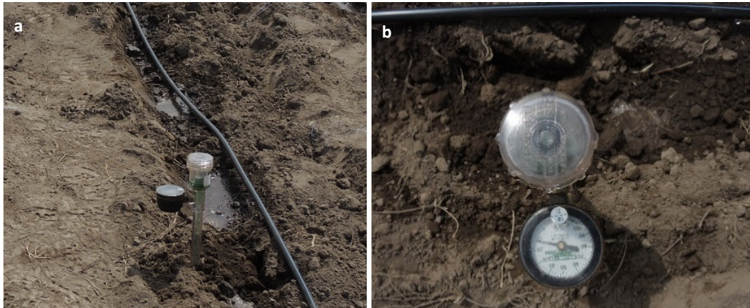
Fig.12 Tensiometer (irrometer®) Installation. a) Lateral and b) front view of tensiometers correct position and location when installed on a field experiment.
