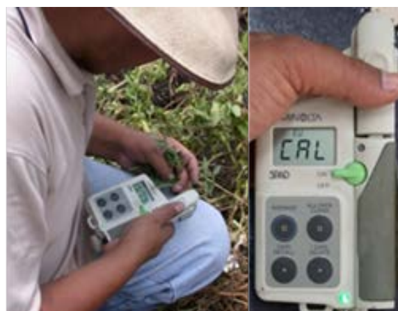
Fig27 SPAD equipment. Showing the correct position of usage to the left; and the calibration option which must be done before use.
