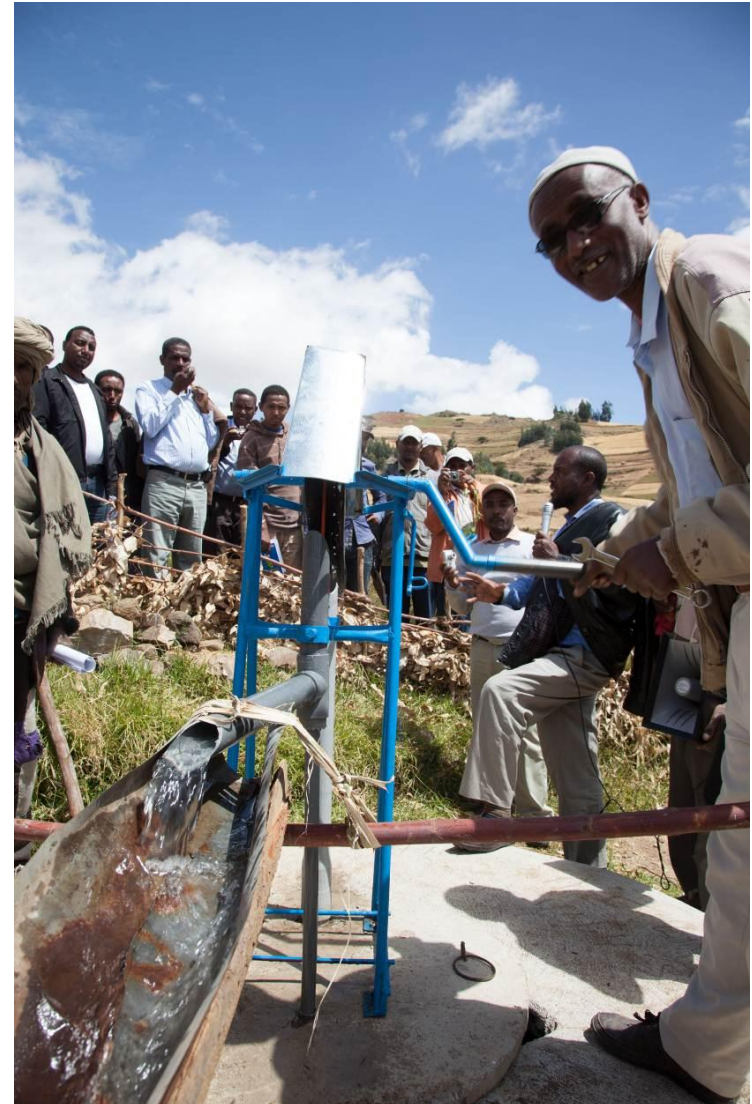
Figure 4. A rope and washer pump installed at a shallow well for irrigation (photo credit: Zerihun Sewnet, ILRI)
