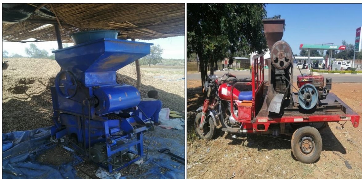
Figure 1: Locally fabricated groundnut (left) and maize (right) shellers in Mwansambo, Nkhotakota, Malawi. Notes: The maize sheller is mounted on a modified Motorbike for ease of mobility to provide door to door services
