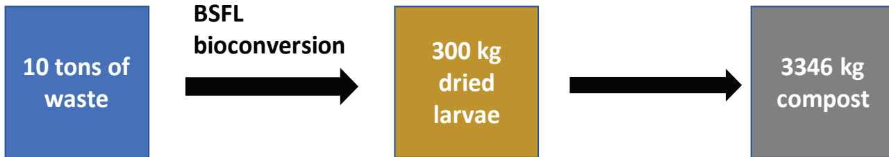
Figure 25b: Efficiency of BSFL biowaste conversion. Depending on the waste type, the stage of larvae harvesting, the initial waste volume can be reduced by 35-66.5 % (wt/wt)
