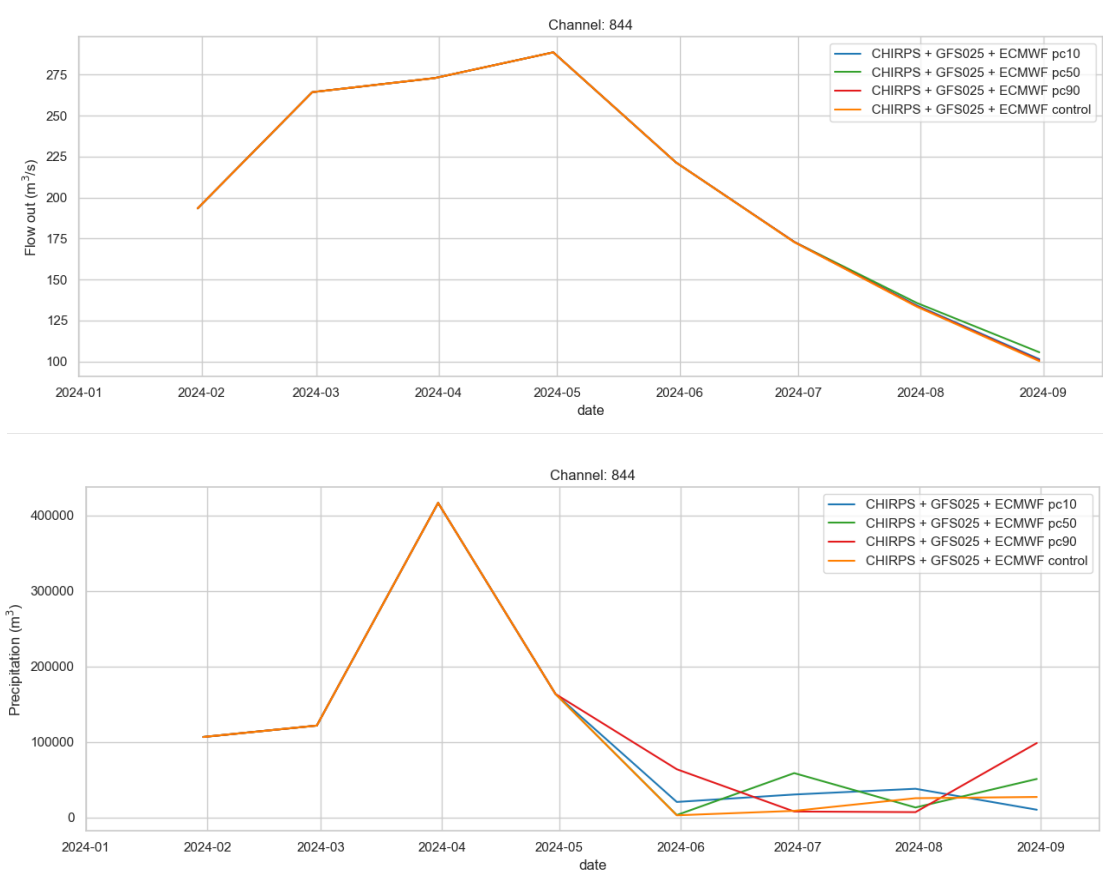
Figure 10 - Flow out and accumulated precipitation for Channel 844 for the SWAT model run with control, pc10, pc50 and pc90 seasonal forecast precipitation. This is the prediction made in 1 of May 2024.
