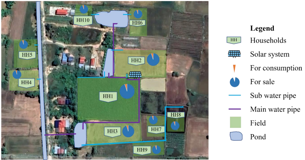
Figure 1. Layout of the SWP system (garden and water pipe locations are indicative)
