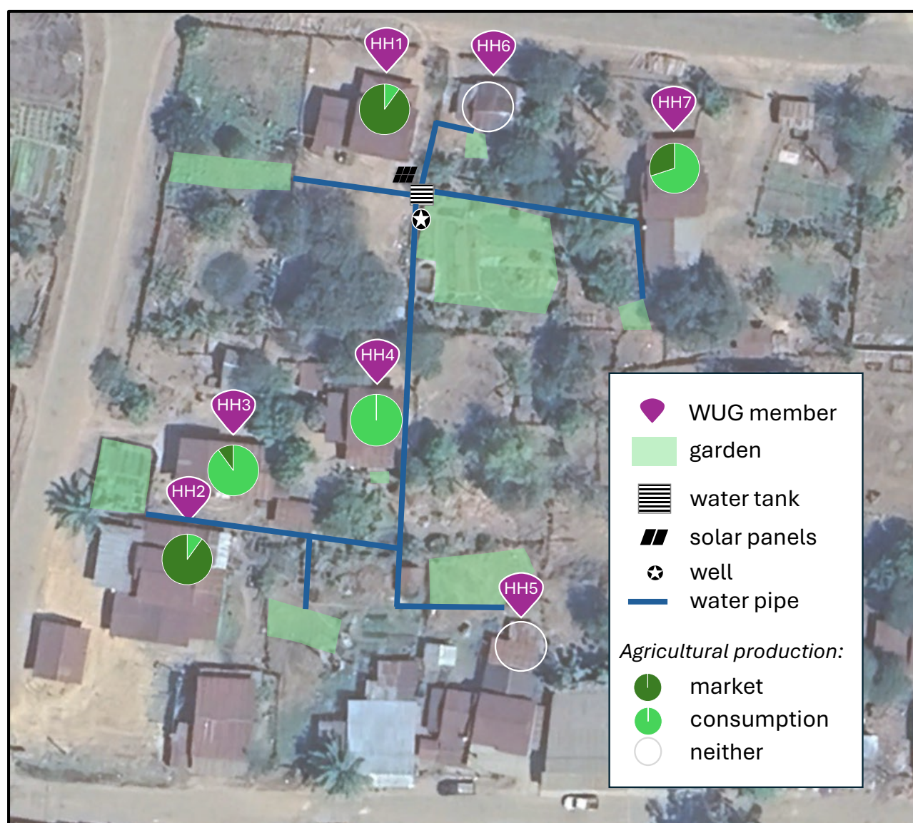
Figure 1. Layout of the SWP system (garden and water pipe locations are indicative)
