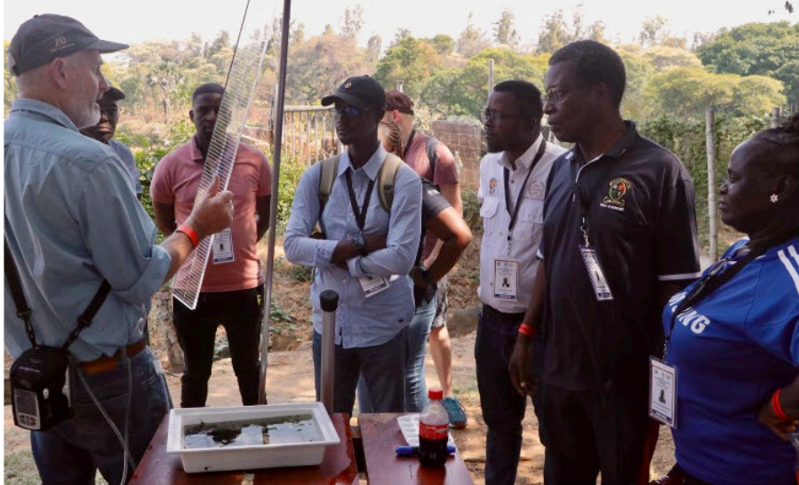
Figure 17. Demonstration of the use of the clarity tube for observing suspended solids in river water, a core parameter of river water quality (photo: IWMI).
