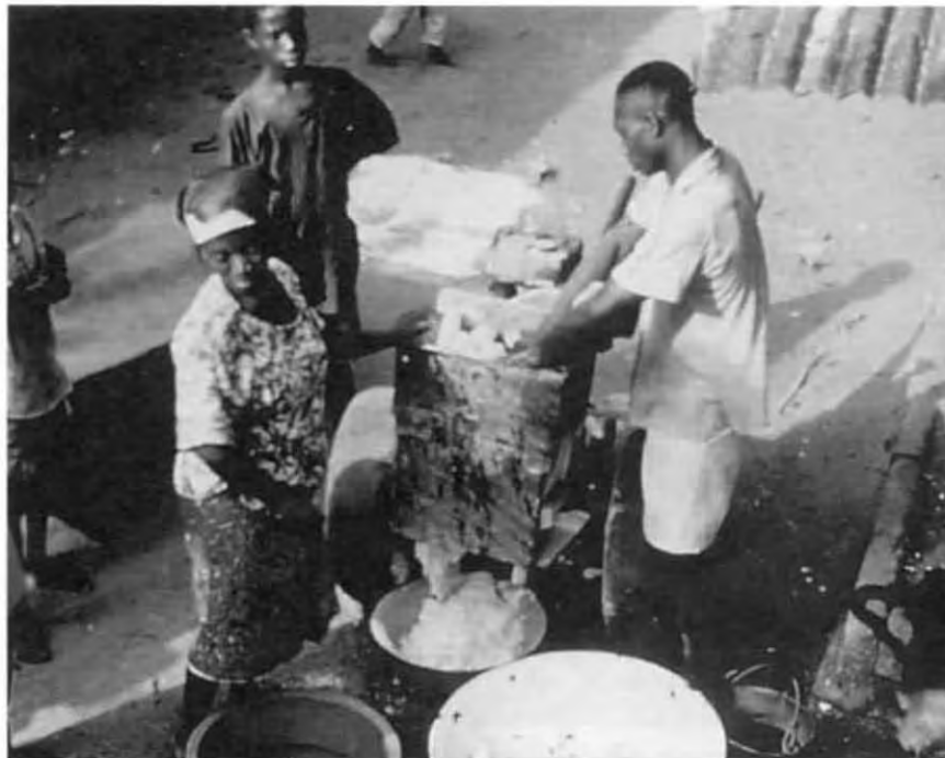
Mechanized grating of cassava for a female farmer in a Nigerian village.
