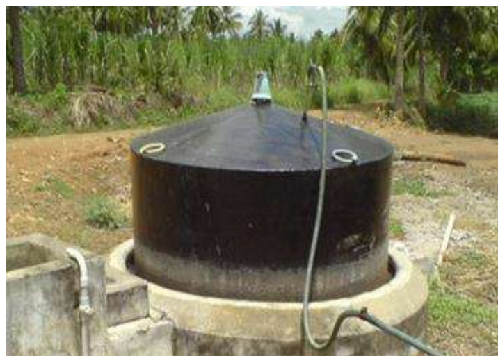
An aboveground biogas reactor; note the pipe used to bleed gasses at the top of the reaction vessel
