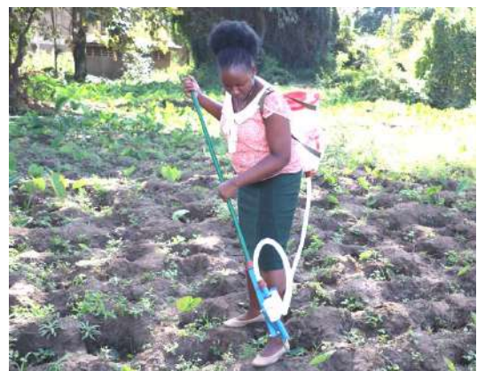
A mechanical device that delivers micro-dosed fertilizers
