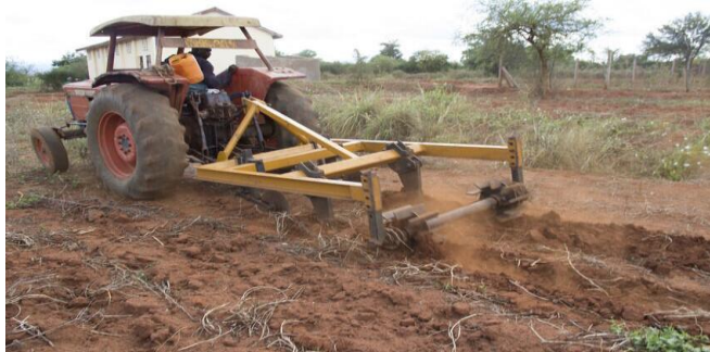
Figure 3: Tractor ripping land.
