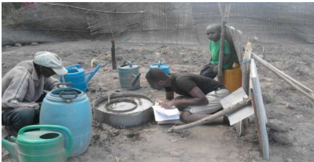
Appendix Figure 7. Infiltration measurement
