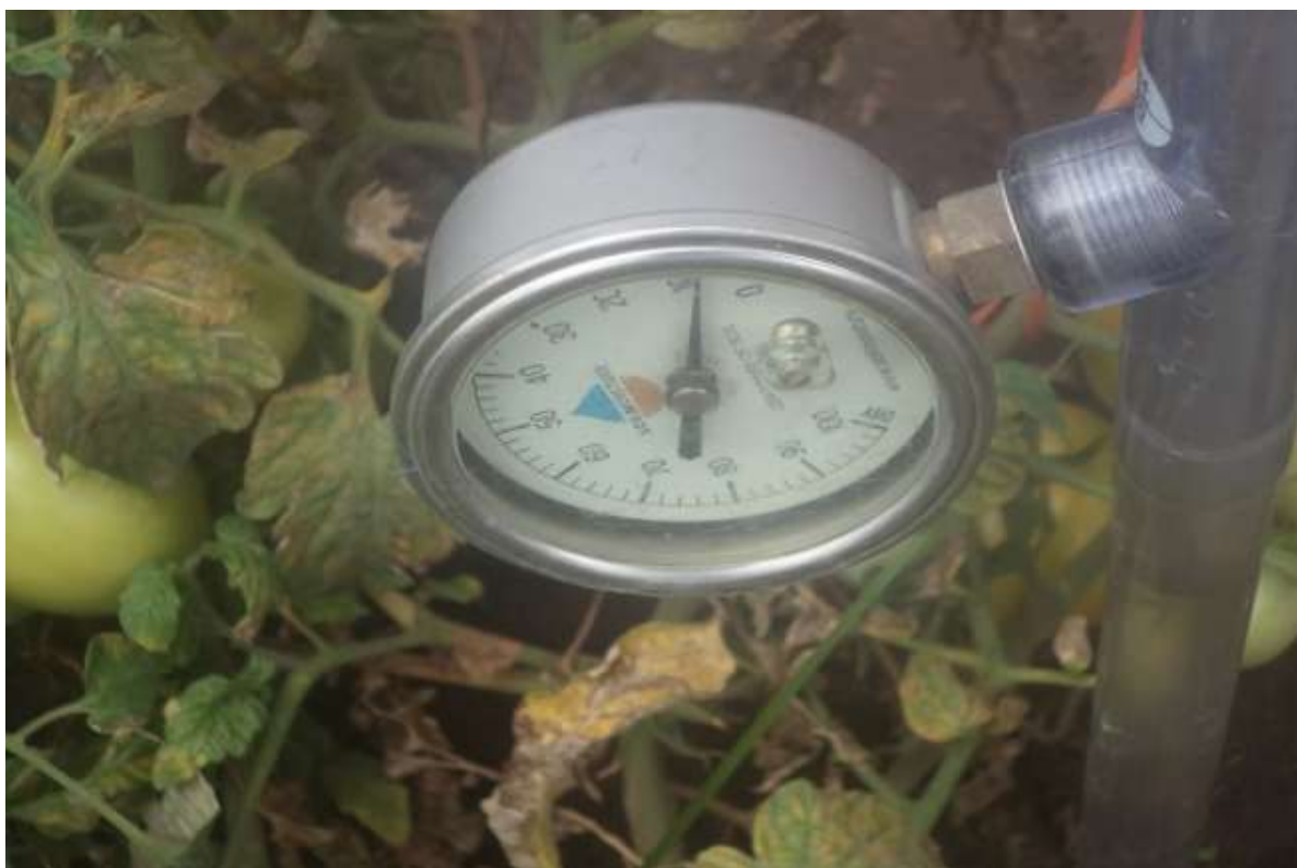
Appendix Figure 10. Tensiometer installed for moisture monitoring at field condition
