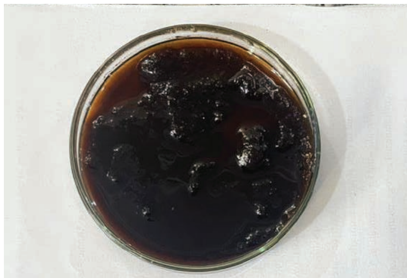
Figure 3. A hydrogel synthesized from rice straw ( photo: Owusu Abebrese, KNUST )
