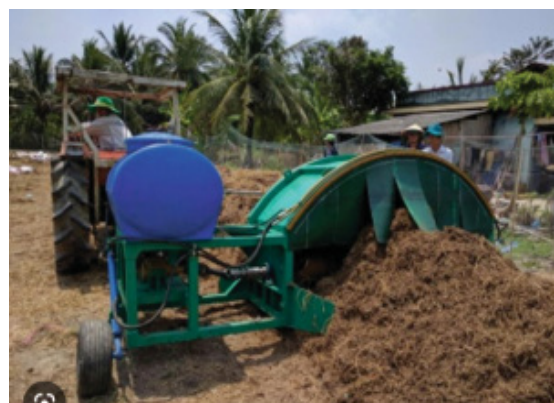
Figure 5b: Equipment for compost turning and watering (tractor and turner)
