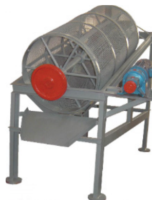
Figure 5d: Compost sieve for sieving finished compost
