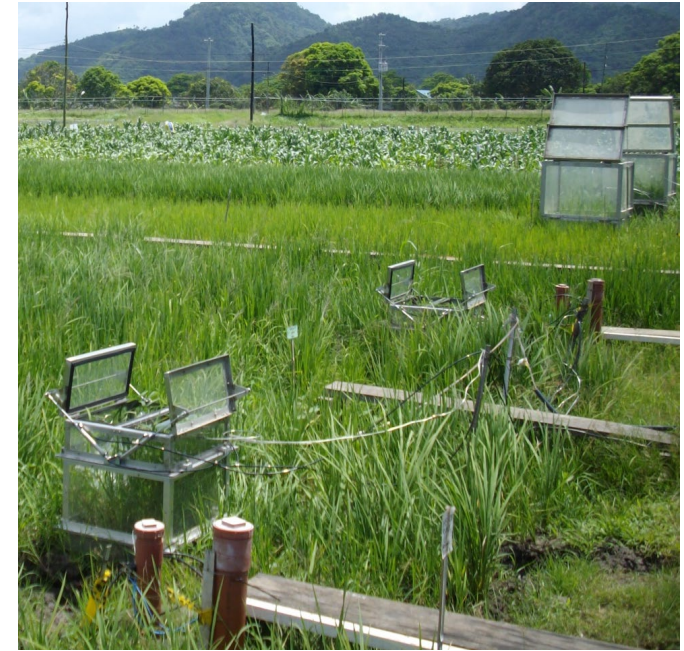
Automated chambers with extension enclosing plants. Los Baños, Philippines
