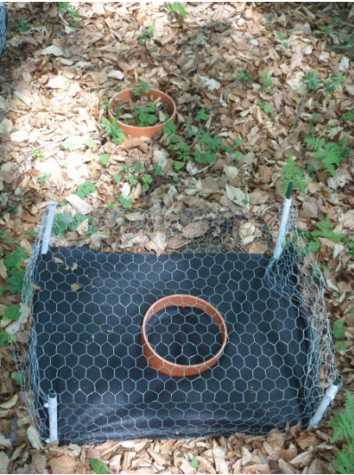
Manual chamber with litter enclosure. Rosalia, Austria
