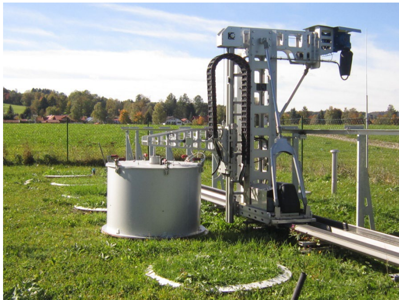
Automated chamber enclosing plants. Los Baños, Philippines
