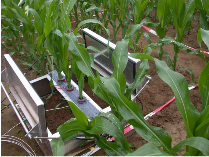
Automated chamber enclosing plants. Los Baños, Philippines
