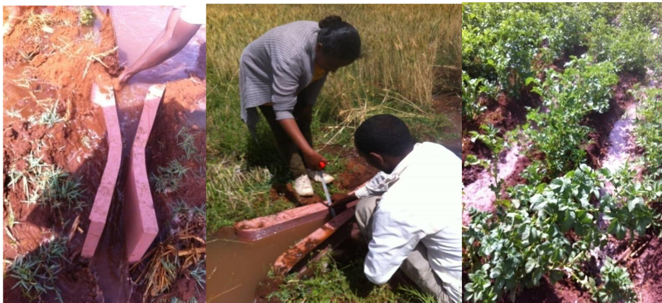
Appendix Figure 2. Discharge measurement by Parshall flume
