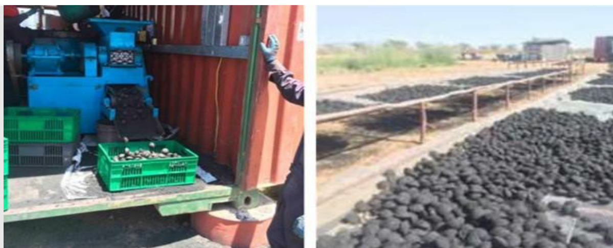
Figure 3: Brikette production in Kakuma Refugee Camp, Turkana, Kenya. Left: Mechanical press producing briquettes from treated sludge and waste biomass. Right: Drying of briquettes (source: Sanivation)
