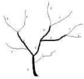
Figure 7-1: Strahler stream order representation
