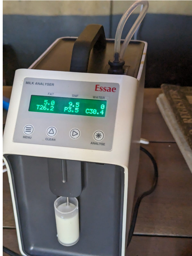
Figure 1: Milk analyzer results during testing showing results for an exceptionally high quality milk sample
