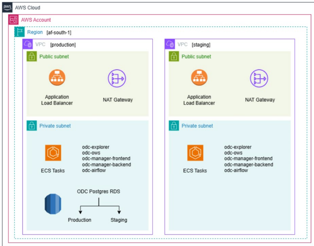
Figure 4 AWS high-level architecture for the Limpopo Digital Twin ODC deployment, showing production and staging VPCs with load balancers, NAT gateways, ECS tasks (odc-explorer, odc-ows, odc-manager-frontend, odc-manager-backend, odc-airflow), and a shared ODC Postgres RDS database. [Source: Authors]
