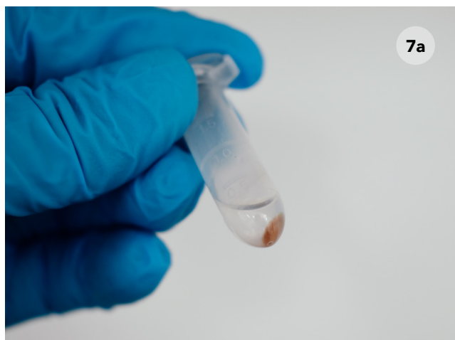
Figure 7. Extract with 0.3 mL of methanol before sonication and vortexing (7a). Extract reconstituted correctly after sonication and vortexing (7b).
