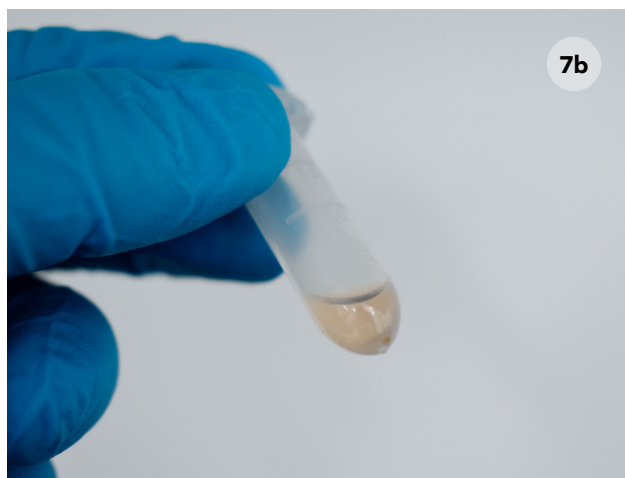
Figure 7. Extract with 0.3 mL of methanol before sonication and vortexing (7a). Extract reconstituted correctly after sonication and vortexing (7b).
