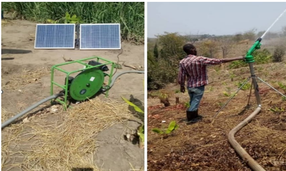
Figure 15. Participant implementing his vision journey using a solar-powered water pump for irrigation. photo: Amon Chinyophiro
