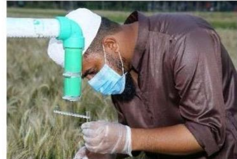
Md. Harun-Or-Rashid is collecting wheat blast samples from a spore trap installed in a wheat field in Jashore. Spores are collected to validate predictions and improve the blast disease early warning system model. Photo: Munim/CIMMYT
